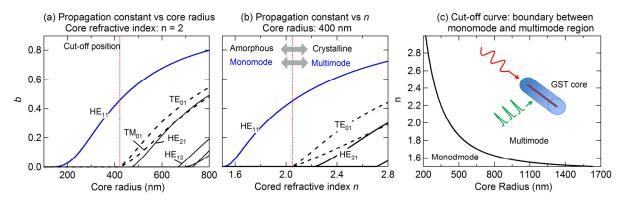
**Fig. 1** Normalized propagation constant as a function of core radius when core refractive index is fixed to 2 (a) and as a function of core refractive index when core radius is fixed to 400 nm (b) for a few low-order fiber modes. (c) Cut-off curve defines boundary between monomode and multimode region.
